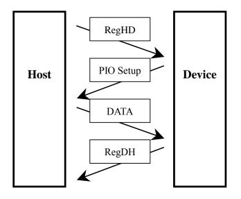
Figure 5.15 PIO data-out command protocol
